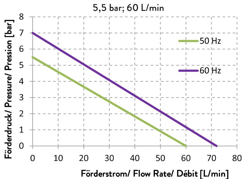
Fig. 105: IN 1030 T, IN 1330 TW, IN 1830 TW
